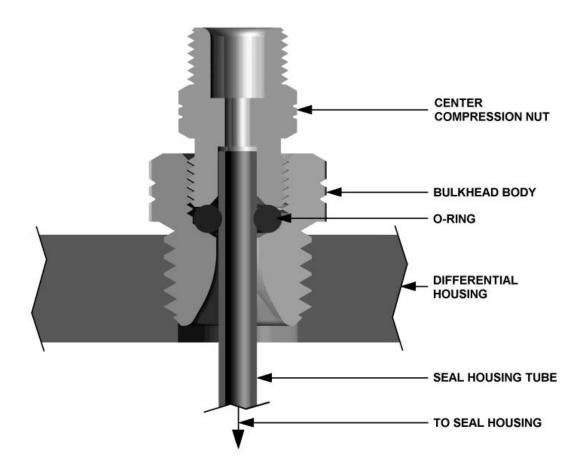
NOTE: Excessive tightening of the center compression nut is not necessary to form a good seal around the tube and may damage the O-ring, the seal housing tube, or the threads of the compression nut.
