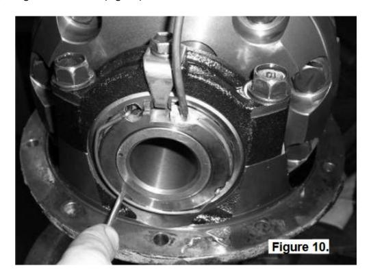
Oheck that the seal housing is now secured from rotating and that it is still sitting flat against the adjuster nut.
