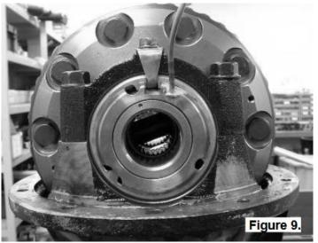
Install the spring clip by first hooking both ends of the clip into the small aligned cutouts of the seal housing and the adjuster nut, and then snapping the clip into the groove of the seal
