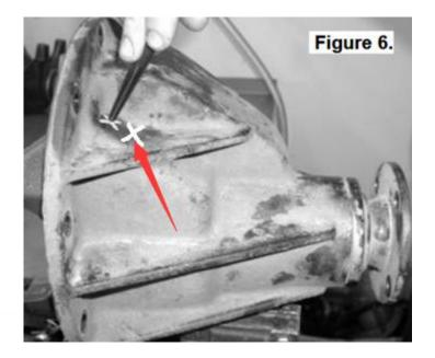
Screw the blue interface bulkhead fitting on the mark of differential case and tighten.
