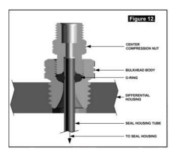
Note : Be sure to insert the correct end of the center compression nut into the bulkhead body. The thread has been partially relieved on the bulkhead side of the center compression nut to visually identify its orientation. (Fig.12.)
