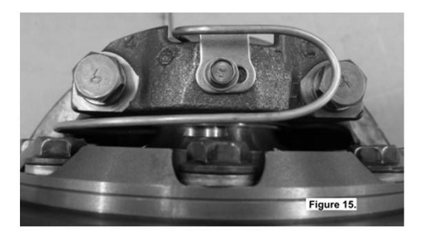
In order for the seal housing to float and self center on the bearing journal, the seal housing tube must not be pulling against the seal housing. To check this, rotate the drive flange back and forth while observing the seal housing movement. The seal housing should rotate slightly against the spring clip, but it should not appear to pull away from the face of the adjuster nut.
