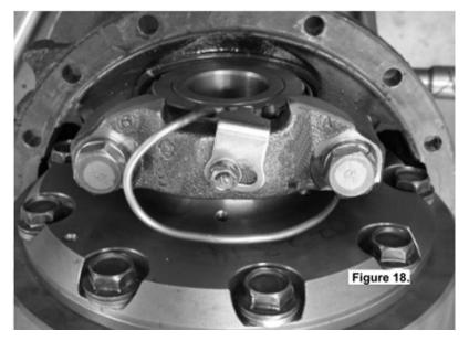
In order for the seal housing to float and self center on the bearing journal, the seal housing tube must not be pulling against the seal housing. To check this, rotate the drive flange back and forth while observing the seal housing movement. The seal housing should rotate slightly against the spring clip, but it should not appear to pull away from the face of the adjuster nut.
