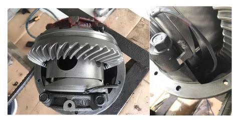
9. Adjust the clearance with the adjustment collar, tighten the fixing screws, and fix the bearing.
