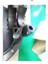
6. Locate the thicker part of the housing where the differential case is facing up. As shown in the figure, drill a hole with a drill of 10.5 and tap the wire of M12\*1.5 on it.
