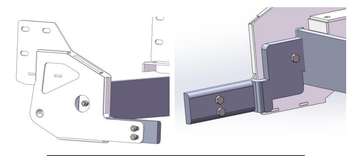
Connect the main bracket with the winch bracket
