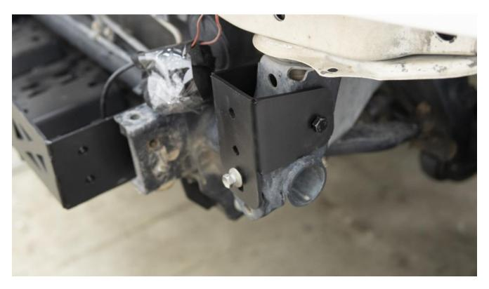
**Step 5:** Install the accessories No. 11 and No. 12 in the diagram of the general accessories and install them on the outside of the fixed points at both ends.
