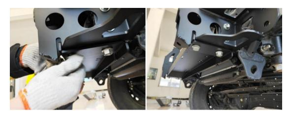
**Step ③:** Install the bullpen on the front bumper (six inner hexagon M10\*25, M10 spacers, M10 flange nuts Tools: T4 Allen wrench, 16 wrench
