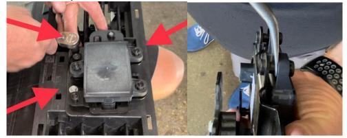
c. Remove 3 gromets from sensor by pushing from front and prying tabs on the back.
