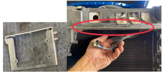
b. Fit the bracket as desired, mark, drill and install with supplied hardware. Then install sensor onto the bracket with supplier hardware & connect to harness.
