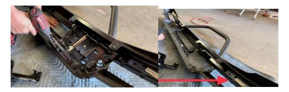
2. Disconnect and remove sensors wiring harness. Remove sensor from plastic retainers by spreading the clip as shown on the backside, and press from the front to the back to remove the sensor. Remove black plastic sensor trim, by pressing the top and bottom tabs on the back side of the bumper, and pushing out of the bumper by pushing back to front. Use of screw driver hand be helpful.
