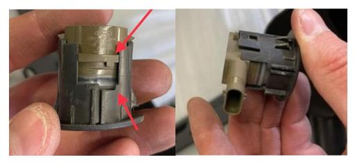
5. Connect wiring harness to sensors. Then proceed to next steps to install the bumper in section 3.
