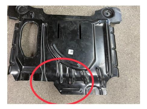
3. 2.7 Engines or vehicles equipped with a transmission cooler will need to trim the bracket as shown below on the driver's side.
