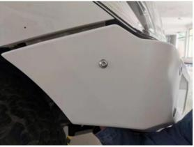
**Step 5:** Install the lower guard plate in Figure 1, a total of 5 screws Figure 2 Install the wheel eyebrow lining bracket, fix the bracket and the bar skin, cut the inner lining according to the fixing hole on the other side of the bracket
