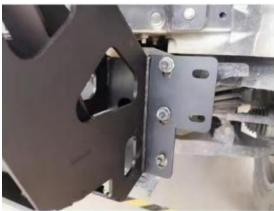
**Step 2:** Install the grid fixing bracket, fix the grid with 3 screws on the left and right, and 4 screws on the triangle bracket in the middle to fix the grid
