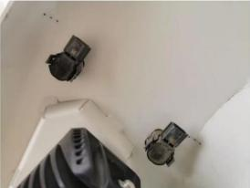
**Step 4:** Install the front bumper skin, fix it with 4 screws on the front, fix it with 2 screws at the guide port of the winch, and fix it with 1 screw on the left and right sides and the corner reinforcement bracket
