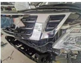
**Step 3:** Install the corner reinforcement bracket and fix the winch tray, fix the bar skin and the corner with 2 screws on the left and right, install the fog lamp, radar probe and wiring harness
